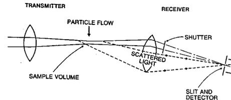
Fig. 9. Schematic of PCSV Sample Volume
