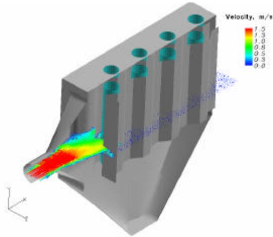
**Figure 10. CFD Simulation. Bags Exit Gas Flow**
