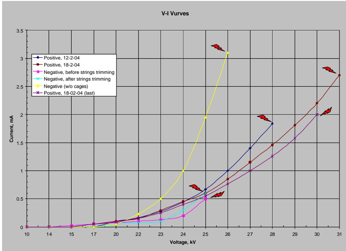
A high-voltage power supply with the ability to provide both positive and negative voltage was utilized to charge the corrugated plates. The goals of these shake-down tests were two-fold. The first was to evaluate the electrical clearances in the pilot-scale unit and to identify any plate/electrode/BFE alignment issues that would result in premature “back corona” or sparking. Once any alignment issues were identified and corrected, the V-I response of the unit was fully characterized.
