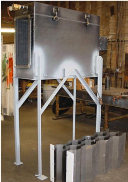
The MSC™ collector is a patented process (Krigmont, US Pat. ? 6,524,369 <sup>(1)</sup>) that entails a unique integration of both electrostatic precipitation and barrier filtration. The MSC™ concept overcomes not only the shortcomings of conventional ESP's and FF's, but is also technically superior to hybrid ESP/FF concepts currently under development. Subsections below will provide the technical background on why the MSC™ concept is a major technological advance in particulate collection.
