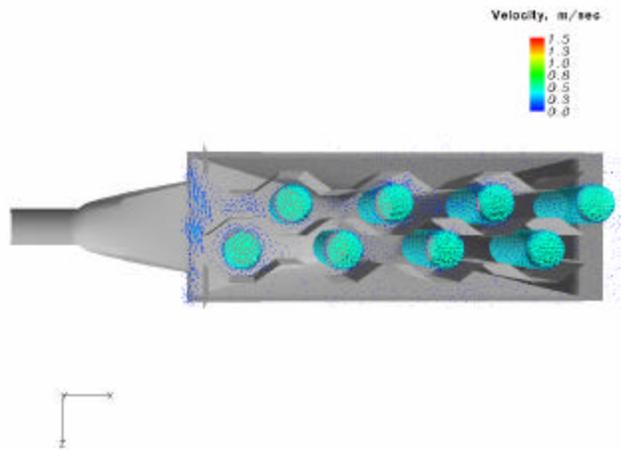
The model included MSC inlet, filtration bags and internal electrodes.
