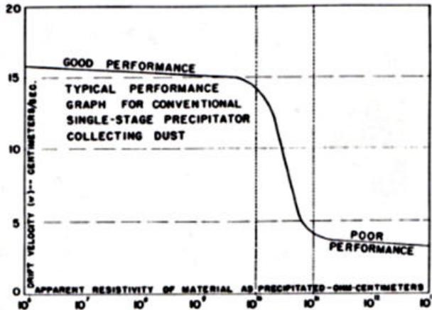
The arrangement of these zones led to two typical precipitator design concepts: (i) a conventional electrostatic precipitator where both zones are combined in a single-stage, and (ii) so called two-stage design where these zones are separated.
