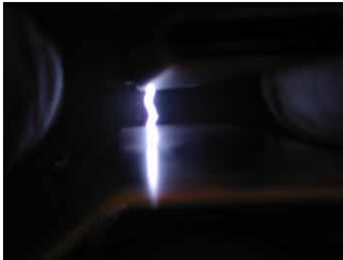
Figure 9. Sparking at the Top of the Electrode System
