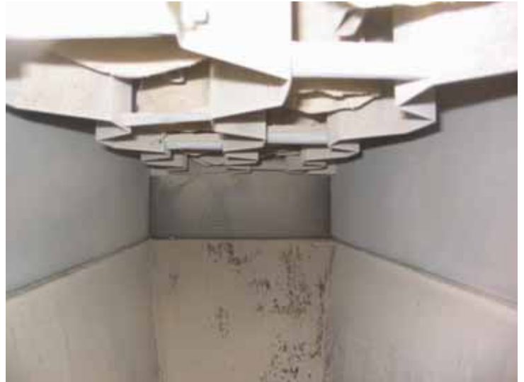
(b) MSC™ Field Energized (27 kV/0.5 mA)
